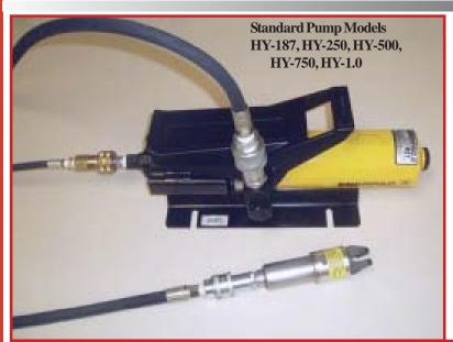
Pinch-off and hermetically seal (cold weld) OFHC Copper, high purity nickle tubing or equal.
